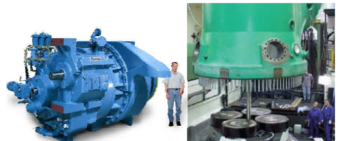
Fig. 3 Worlds largest operational wind gearboxes. Left: Winergy 5MW gearbox. Right: Renk 5MW gearbox (during assembly).
