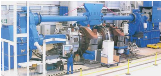
Fig. 6 Back to back testing of multimewatt gearboxes [14]
