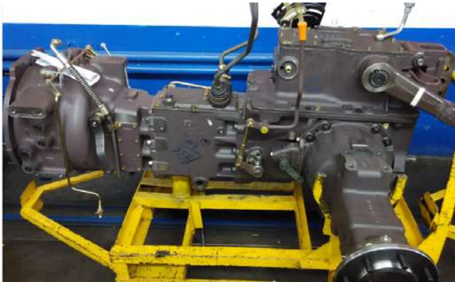
Figure 1.1-2: Transmission with rear axle and motor mount ready for final assembly.
